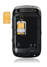
Slide the SIM card into the slot.
